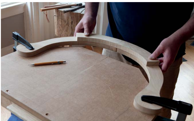
Glue the doubler to the arm. Clamp the pieces together whilst the arm is clamped to your alignment board.
