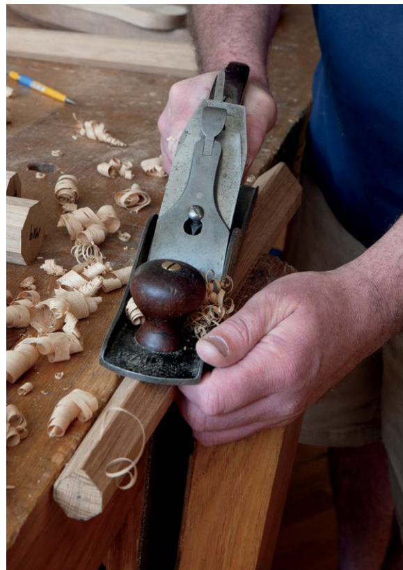
Shape the legs to a tapered octagon with a jack plane. The leg vice is helpful as it clamps tapered shapes easily.
