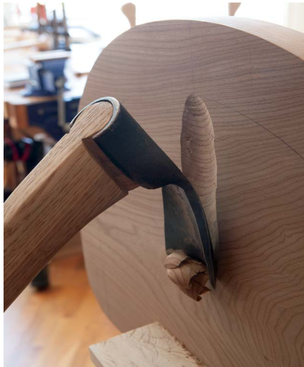
Note the wooden guard below the adze. It protects the vise jaws and adze's edge from damage.
