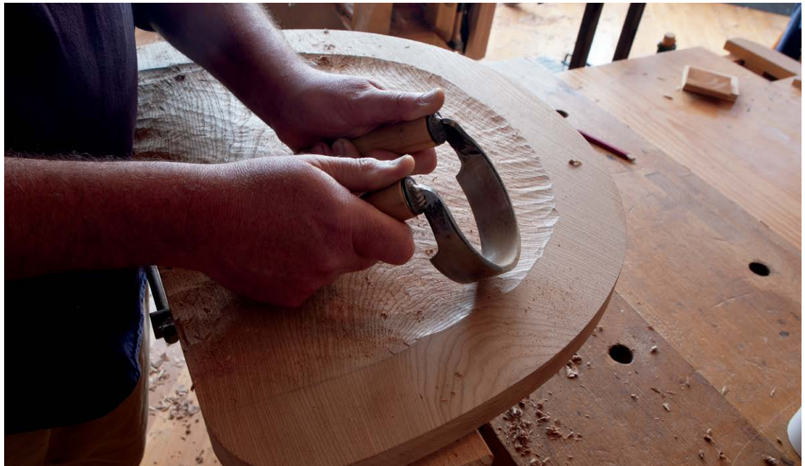
The scorp removes the high furrows left by the adze and further refines the shape of the saddle.
