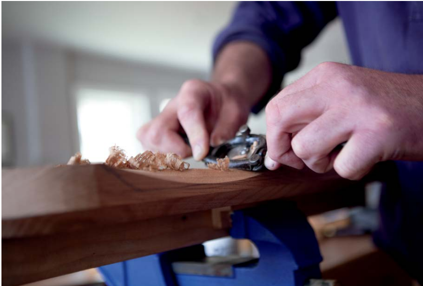
The No. 53 spokeshave is the ideal tool for shaping the concavities at the front edge of the seat.
