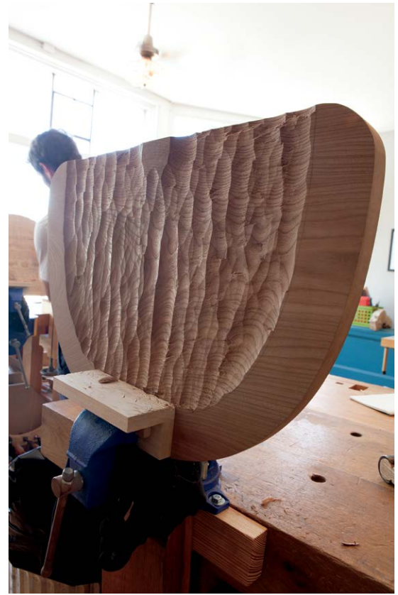
The finished saddle after a few minutes of work with the adze.
