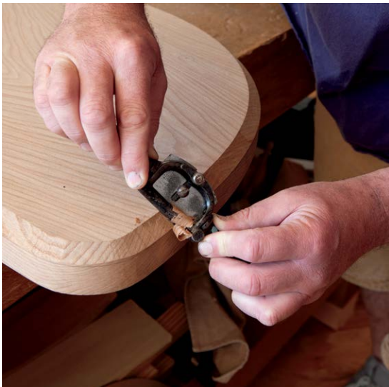
After sawing the bevel on the underside of the seat, clean up the cut with a spokeshave.
