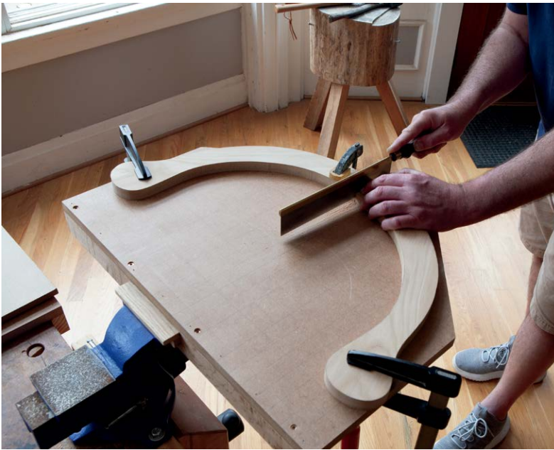
Press the two ends of the arm together and then saw through the joint. Repeat until the joint closes tight.
